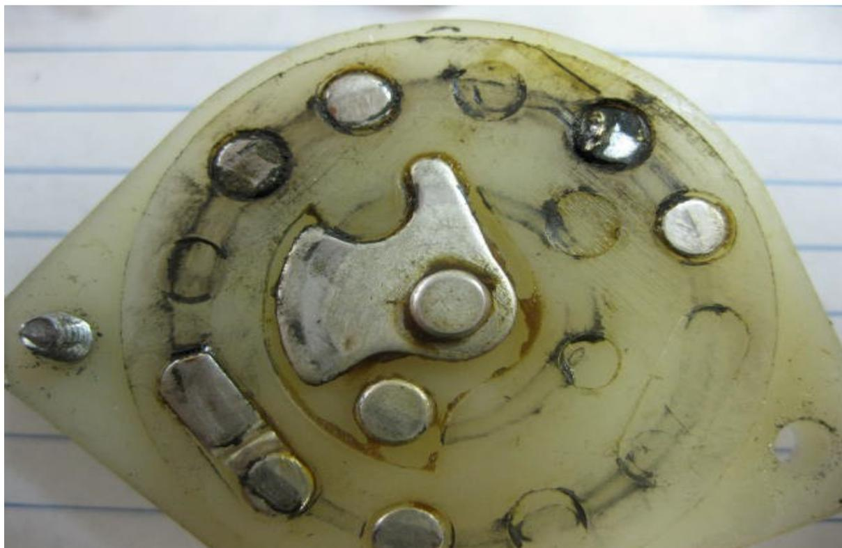
**Cessna 172S, Failed Ignition Switch, ATA 7430**
